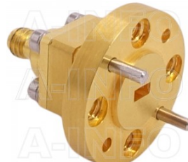
12WECA1.0_Cu Endlaunch Rectangular Waveguide to Coaxial Adapter 60-90GHz WR12 to 1.0mm Female
